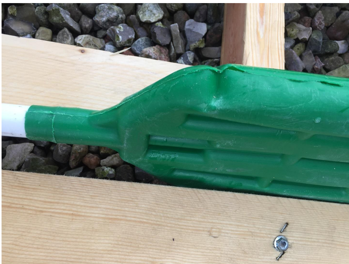
Figur 6. Paddel, der er revnet, kan ikke garanteres ren indvendig og skal kasseres (iflg. DANISH Transportstandard). Paddle that is cracked cannot be guaranteed to be clean on the inside and must be scrapped (according to DANISH Transport Standard).
