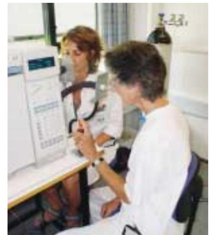
Gas chromatograph with mass spectrometry (GC/MS). As a novelty, the GC/MS at the Danish Meat & Research Institute has been equipped with two odour gates. While the individual substances from the housing unit air are being analysed at mass spectrometry, two persons can smell the same substances individually and describe the intensity and the characteristic odour concentration of the substances.
