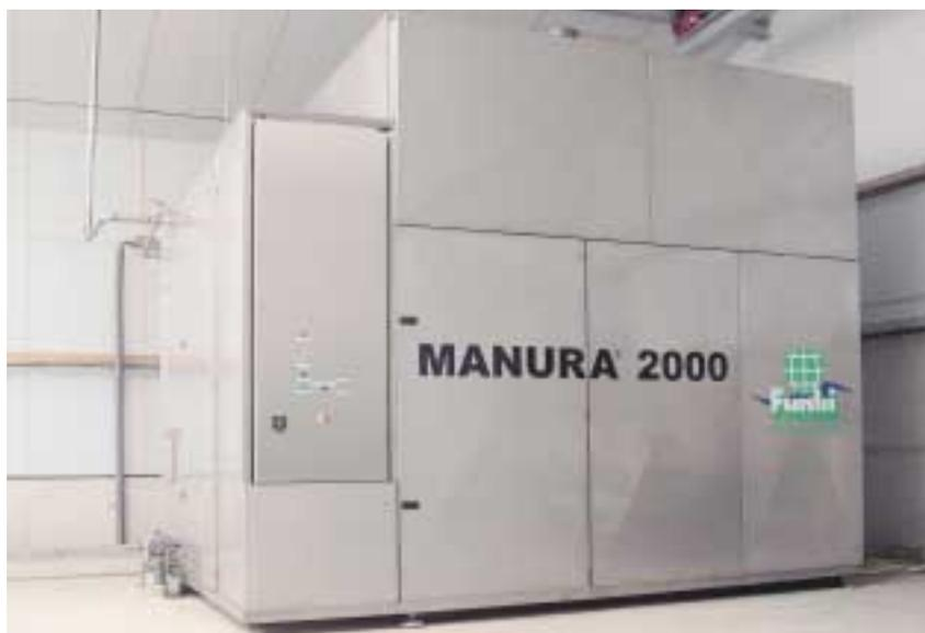
The Funki MANURA Compact belongs to the high-technological group. The slurry is separated into concentrated nutrients and "pure" water.
