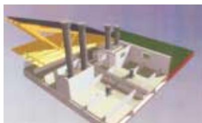
*The system from Perstrup Betonindustri and Skov A/S transfers the outlet air via floor exhaustion to the biological purification system, where the air passes through the bacteria-coated lamellas.*
