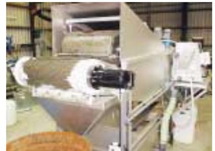
*Ansager Sep Tec: flocculants are added prior to separation on a belt.*
