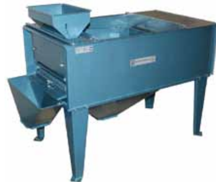
Pig Research Centre tested three different grain cleaners: results showed that cleaning ability did not differ. The above screen cleaner from Øgendahl Maskinfabrik was one of the three tested cleaners.
