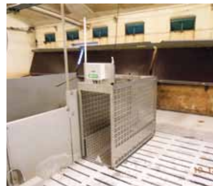
Figure 2 – Pigs are automatically weighed when they pass through the scale.
