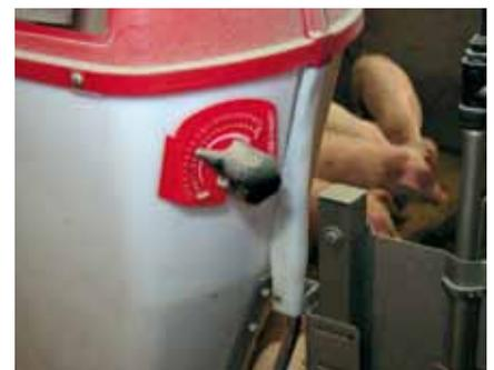
*A clear scale and a simple method for setting the feeder.*
