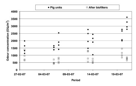
Figure 2. Odour concentration in the air from the pig units before and after it has passed through the biofilters.
