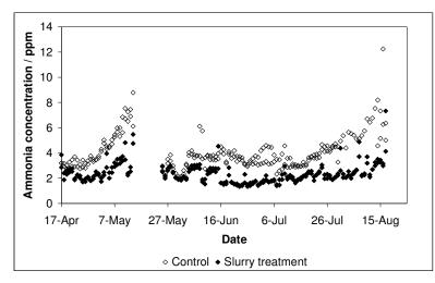
Figure 2. The daily average ammonia concentrations in the exhaust air from the four experimental sections with and without treatment of the slurry
