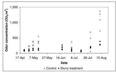
Figure 1. Odor concentration in the exhaust air from the four experimental sections with and without treatment of the slurry
