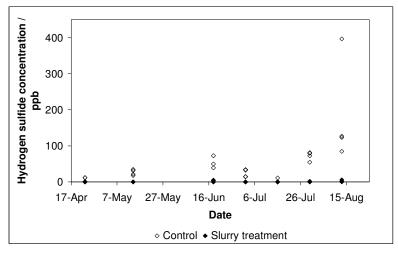
Figure 3. Hydrogen sulfide concentrations in the exhaust air from the four experimental sections with and without treatment of the slurry
