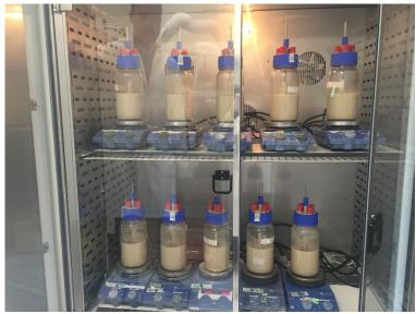
Photo 2. Fermentors used in the laboratory trial (photo: Nuria Canibe).
