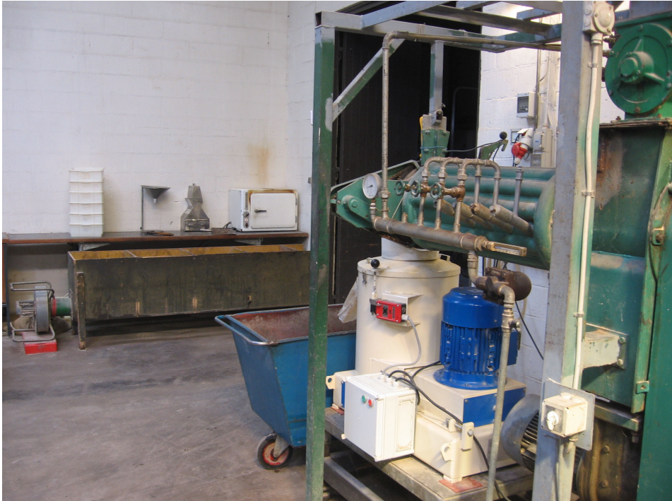
Mini feed mill with ventilator, cooling box, pellet press, steam and cascade mixer
