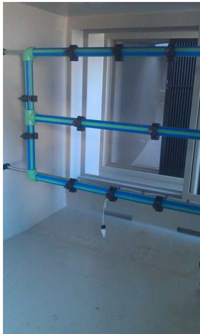
Figure 3. Nozzle bar that moisturized the air using sulphuric acid mixed in water.
