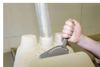
Cleaning and setting of feeders
