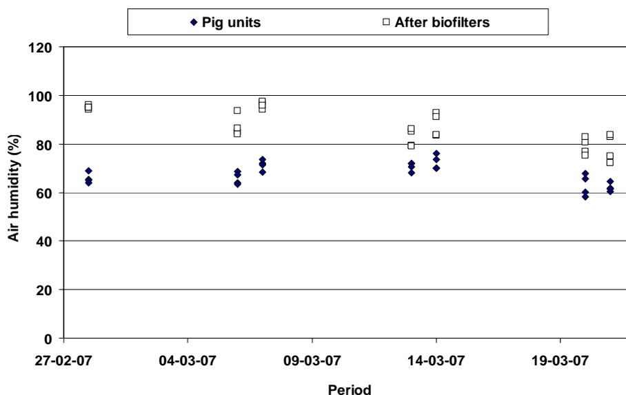
Figure 4. Relative humidity in the air from the pig units before and after it has passed through the biofilters.
