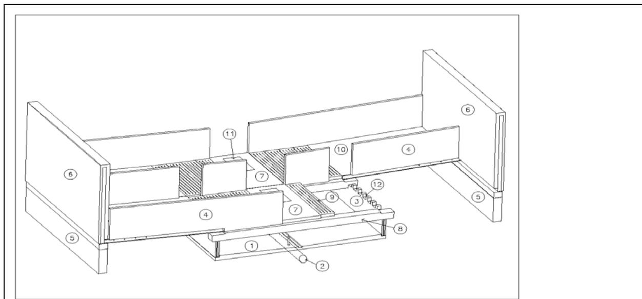
**Figure 1.** Drawing of the Perstrup pig house with pens with partially slatted floor, sloped manure channel with a gutter for urine drainage and partial air evacuation directly from the manure channel through a ventilation channel under the solid part of the pen floor.
