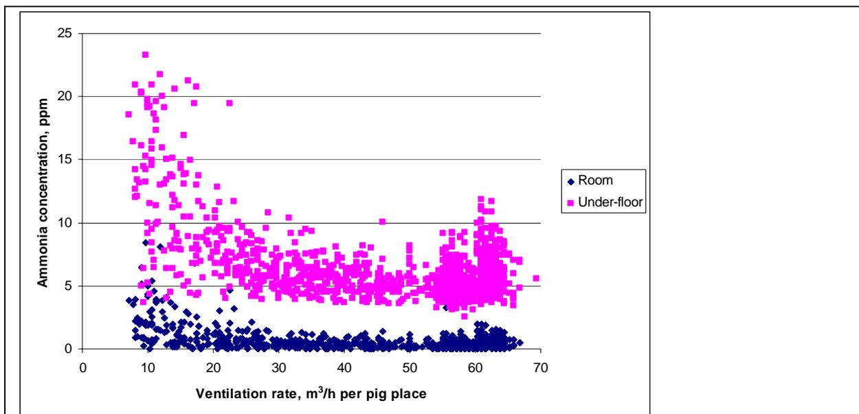
**Figure 2.** Measurements of ammonia concentrations in the room and under-floor respectively depicted in relation to the under-floor ventilation rate. The measurements originate from the first batch in the control unit April to June 2007.
