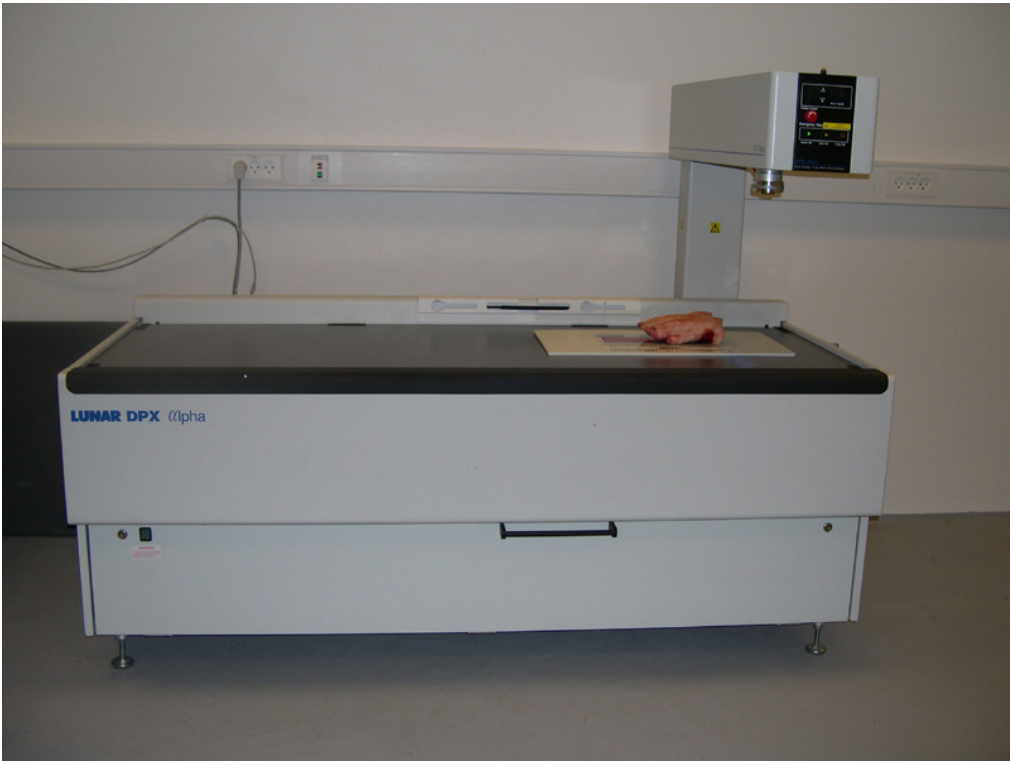
Figure 2: Scanner for DEXA scanning of bones
