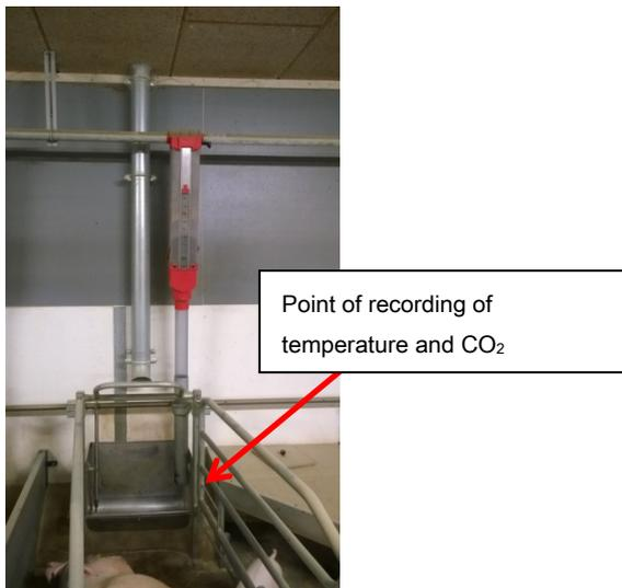
Figure 2. Location of temperature and CO<sub>2</sub> sensors. The sensors the placed at the end of an iron tube to protect sensors and wires.
