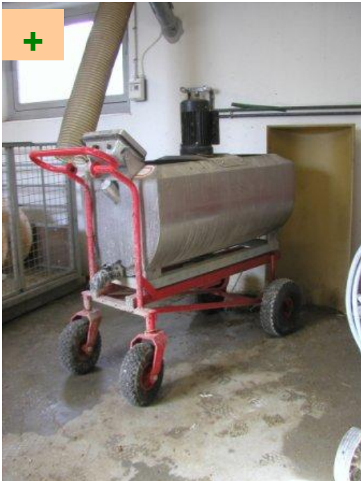
Feed cart for feeding of gruel feed. The weaner diet is given as dry feed or liquid feed / gruel feed.
