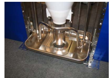
Water circulates past nipple drinkers (via cross pipe fitting)
