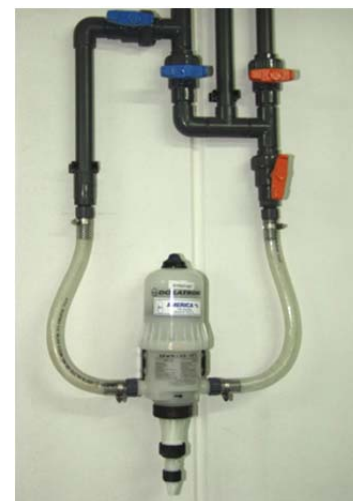
Medicator is connected to the section/pen housing pigs to be treated
