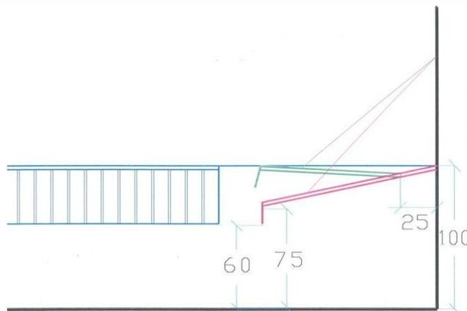
The effect of removing the front edge on the upper images can be compared with raising the cover with fixed front edge as in this figure. The open area towards the pen is not increased quite as much by raising the cover as shown in the images above. Put roughly, the change illustrated in the figure may reduce the temperature by 3-4 degrees in the creep area. Once the lid of the covers is raised above the pen partitions, open up completely to avoid chimney effect.
