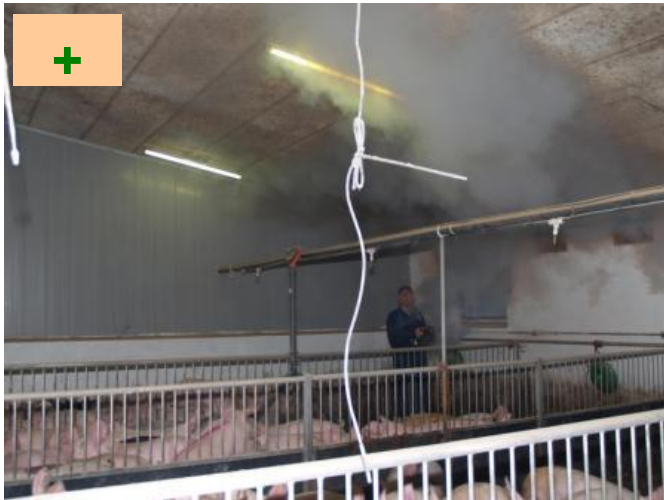
1. Smoke is used to check air flow
